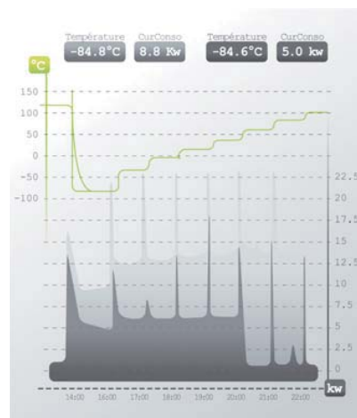
This standard test cycle clearly shows the energy saved with the "Energy saving" cycle (dark grey curve) compared with a cycle without this mode (light grey curve). Electrical consumptions are displayed instantly.
