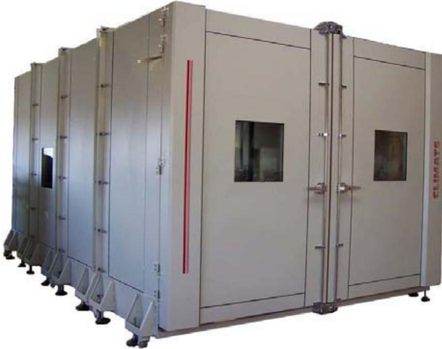
Climatic chamber of large capacity (26 m<sup>3</sup>) made up of 4 rings.
