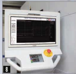
8 Oven process control system
