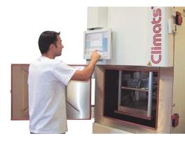
All of our environmental test chambers are controlled by the software **Spirale** 3
